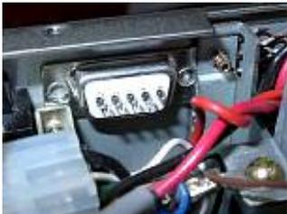
Connect the DB9-pins to the relay outputs of the band decoder using flat ribbon cable. Ground connection is made via the metal case of the DB9 connector. Remember to connect the case of the DB9-plug to ground.
