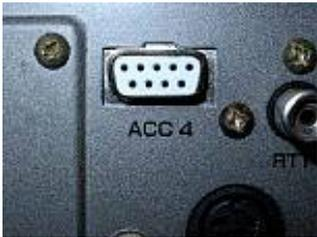
Loosen all screws of the rear panel. Remove the 3 screws that hold the RTTY/DSP1/DSP2 connector board
