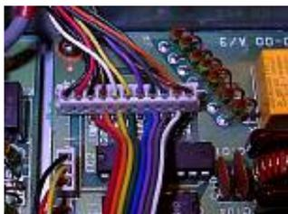
Solder 9 wires of a 10-wire flat ribbon cable to the pads and connect to the corresponding inputs (33K resistors) on the band decoder board. The remaining wire is connected to +12V as supply voltage for the relays. Use a separate wire for
