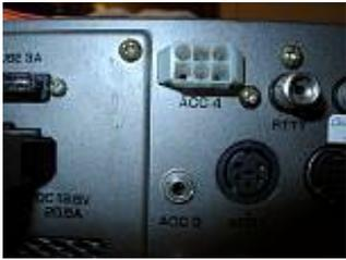
I used a DB9 female connector for the relay output signals. The connector can be mounted by replacing the ACC4 connector which is provided for connecting the external antenna tuner AT-300. You won't need this connector with the build-in automatic tuner. Just remove the ACC4 connector and push it back into the case.
