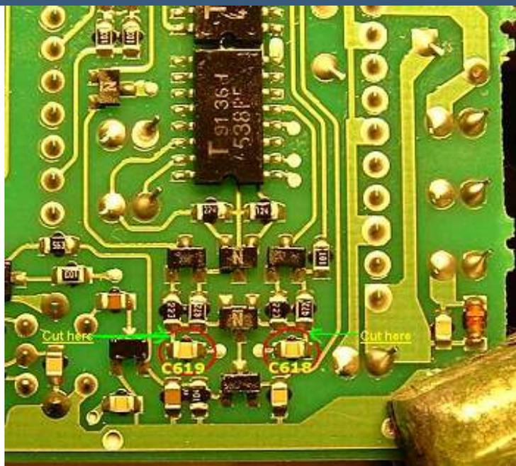
The capacitors to isolate are C618 and C619
