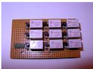
My circuit uses 9 miniature relays (12V DC, spst type) to drive any remote antenna switch. The relay contacts are switched to ground when active (see circuit diagram) but it's also possible to switch to +12V if needed.
